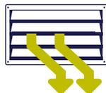
To avoid potential issues, leave your vents or registers open in all rooms, even when you aren't using them. Closing them can cause air pressure problems for your ducts, and closed vents can lead to irregular airflow and increase the risk of costly breakdowns.
